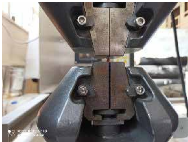
Figure 1. The Mechanical test devices; Shimadzu 100kN static tension-compression test devices.
